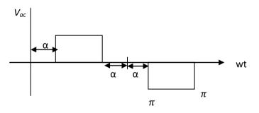
Fig 1: Inverter output for amplitude and harmonic control
